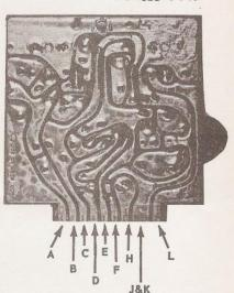
Note: All measurements made with the VOX removed from the set, using a Hewlett Packard VTVM #410B. DO NOT use a VOM for measurement. Setting of the controls of no importance. Measurements made from terminal K as a common point. Some variation may occur with various settings of meter range switch of #410B.
